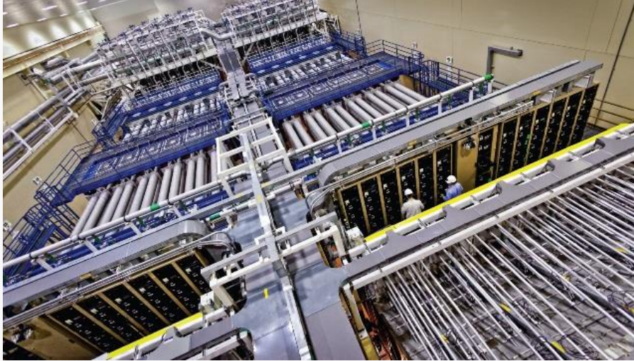
NIF Laser Bay 1, showing a portion of the 192 laser tubes heading to the target chamber
